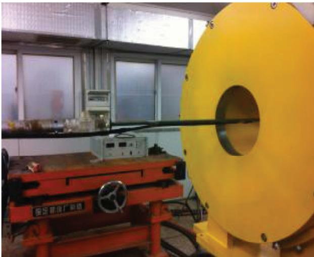
Figure 4: The Measurement of radial magnetic field. The data of the radial magnetic field is shown in Figure 5.
