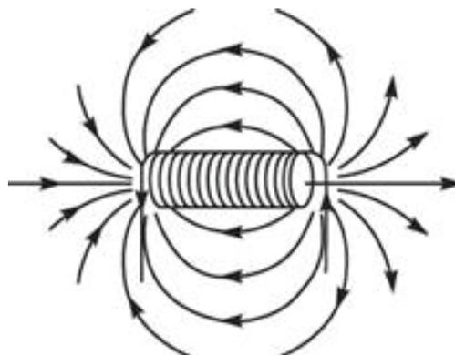
Figure 2: The Magnetic field distribution of Solenoid Magnet.
