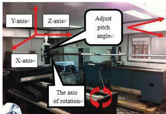
Figure 1: Hall-Probe Measurement Facility.
