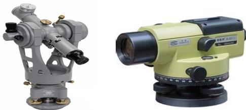
Figure 4: The Theodolite and Level.
