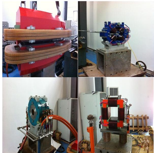
Fig.1 Four types of magnets (Note:From left to right, first line, the dipole magnet, the quadrupole magnet; second line, the solenoid, the correction magnet).
