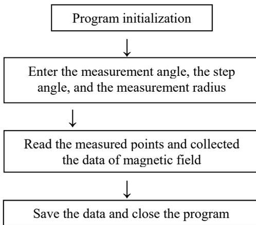
Figure 2-a: The program flow diagram.
