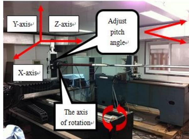
Figure 3: Hall-Probe Measurement Facility.
