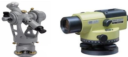
Figure 4: The Theodolite and Level.
