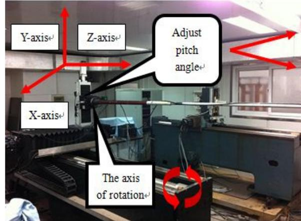
Figure 3: Hall-Probe Measurement Facility.
