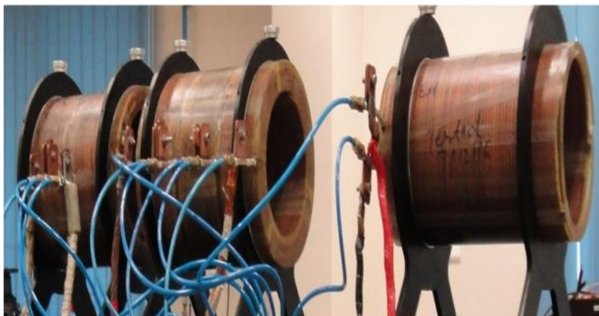
A set of three water cooled solenoids (L) and their combined field profile (R).
