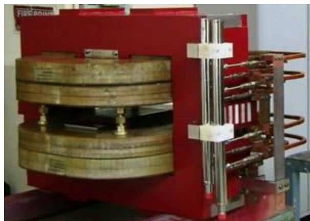
H-type Dipole magnets for CLIC test facility, CERN.
