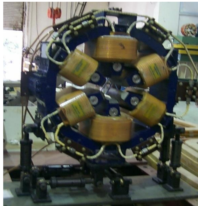
Indus-2 sextupole magnets (Wt. \sim 0.6 MT) with support/positioning system (Right).
