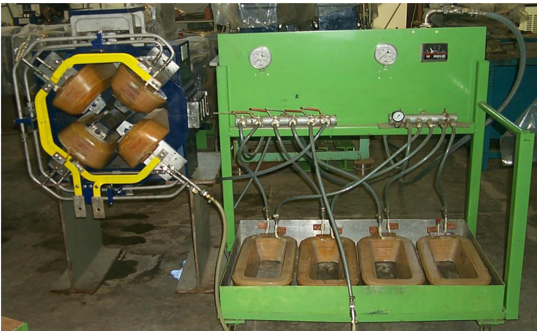
Hydraulic-Pneumatic test set-up for water-cooled QP magnet coils
