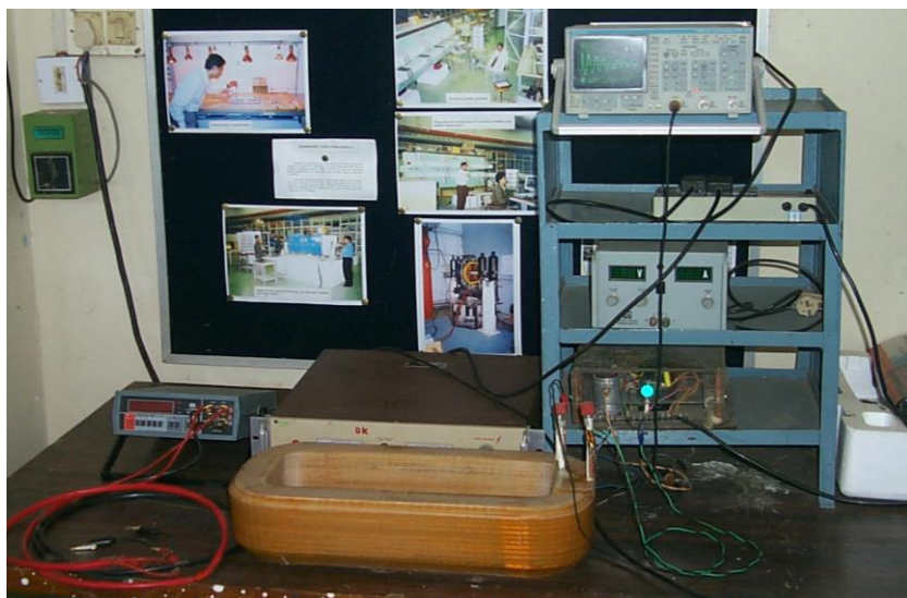
Electrical test set-up for magnet coils
