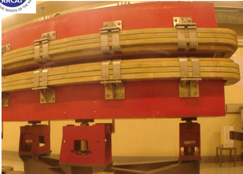
Support system mounted below the Dipole magnet
