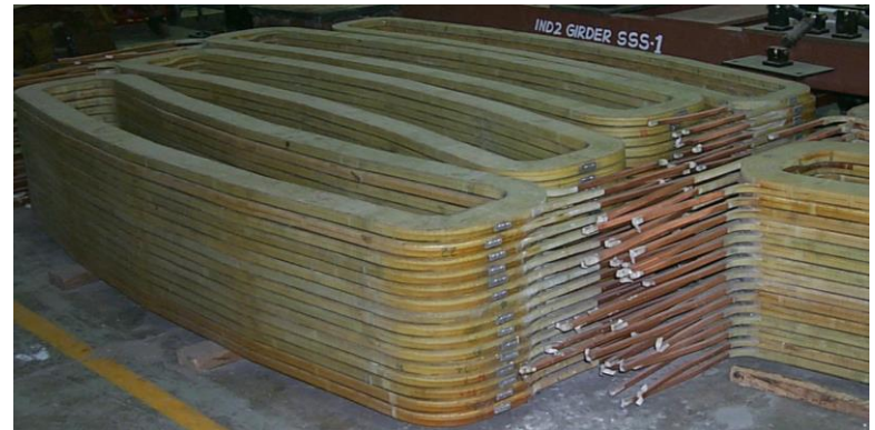
Dipole magnet coil winding machine and epoxy-resin encapsulated coils .
