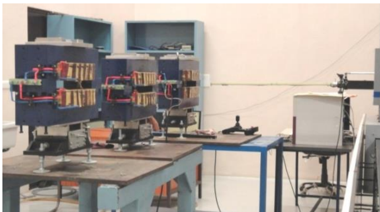
Dipole magnets in measurement bench.
