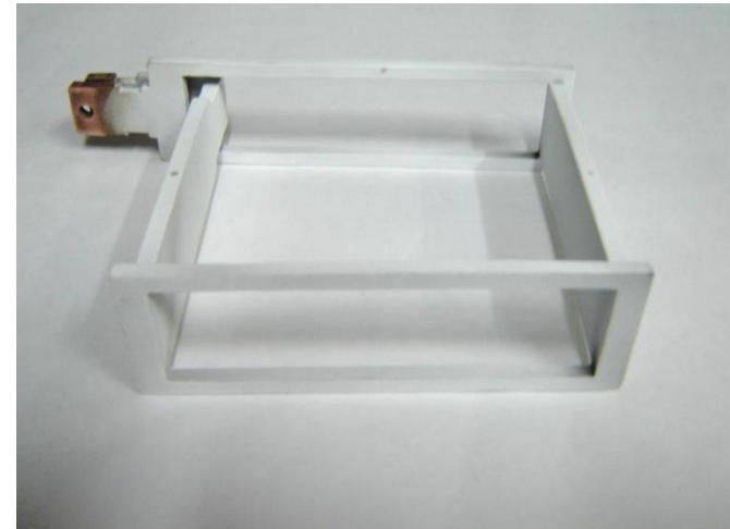
Alumina coated copper coil for kicker magnet.
