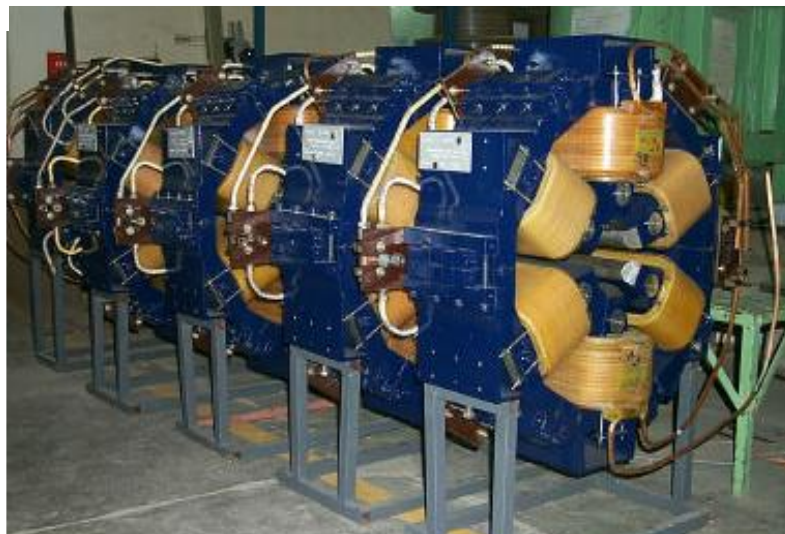
Indus-2 sextupole magnets (Wt. \sim 0.6 MT) with support/positioning system (Right).
