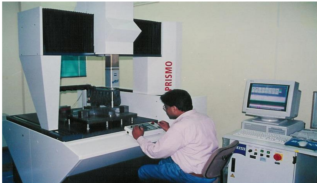
Inspection of core laminations on co-ordinate measuring machine
