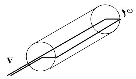
$$\begin{split} V &= \partial \Phi / \ \partial t = N_{coil} A_{coil} \ \partial B_r / \ \partial t; \\ &= N_{coil} A_{coil} \sum_{n=1}^{\infty} \left\{ \!\! n^2 r^{n-1} (A_n \sin n\theta + B_n \cos n\theta) (\partial \theta / \ \partial t) \right\} \end{split}$$
