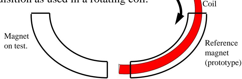
The coil (with multiple radial windings) is traversed from the reference to the test magnet; voltage from each winding is integrated; variation from zero in the integrated volts, after the traversal, indicates variations from the reference magnet total flux vs radius values, which are known.
