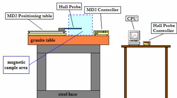
Figure 2: Diagram of the mapper's main parts.
