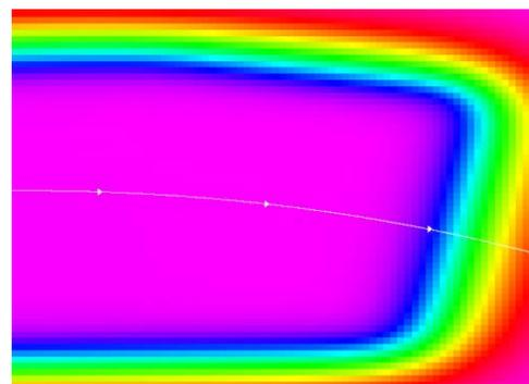
Figure 5: The orbit of an electron in the B-field of a bending magnet.
