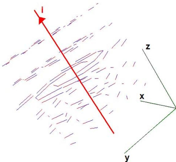
Figure 6: Linear current's reconstructed field.
